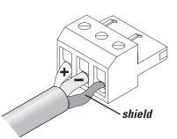
Terminal block: balanced connections
